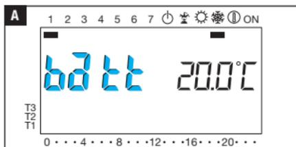
The letters **batt** on the display means that the batteries are flat and must be replaced.
