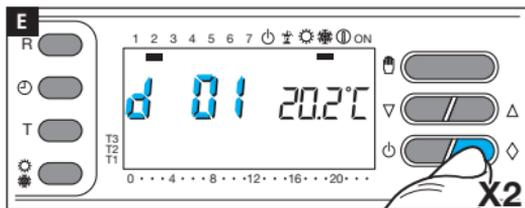
Use buttons  $\nabla/\Delta$  to set the desired number of days of activation (from 1 to 99) **F**.
