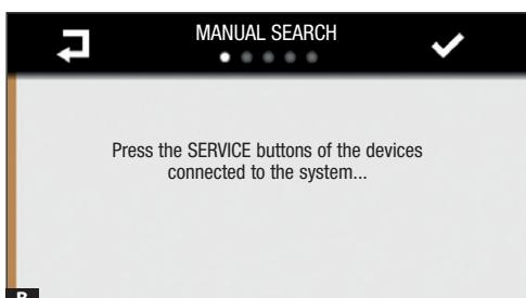
Press the 'SERVICE' button found on all devices connected to the BUS. On the TA/P1 zone thermostat, instead of the 'SERVICE' button, simultaneously press the buttons .
