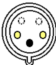
3-pole +N+PE 380V-415V AC red
