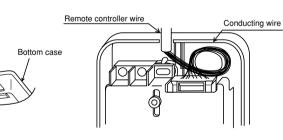
(6) Install the lower case on the switch box or directly on the wall.
