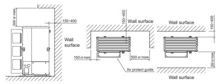
2) Multiple unit installation: \* Installation of multiple units in series must be no more than five units.
