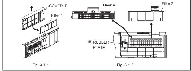
2. Remove the filter from the indoor unit. (Fig. 3-2)
