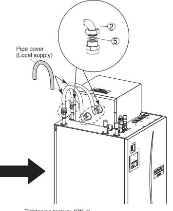
Tightening torque: 42N·m Use double spanners.
