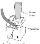
Do not insert more than one connecting cable into each terminal of TB571 and TB530.
