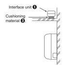
\* When mounting the interface unit 1 using a cushioning material 3, be sure to mount it in a location where it will not fall.
