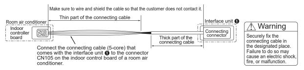
• The connecting cable (5-core) connected to a room air conditioner should be wired according to the room air conditioner installation manual.
