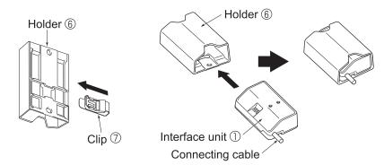
Slip the clip ⑦ over the edge of corner box to fix the interface unit ①.
