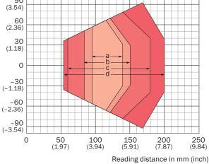
For devices with plastic reading window, the depth of field is reduced by approx. 10 %.
