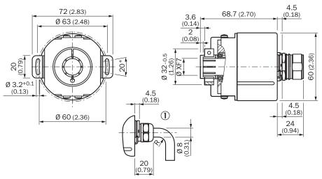
General tolerances according to DIN ISO 2768-mk ① R = min. bending radius 40 mm
