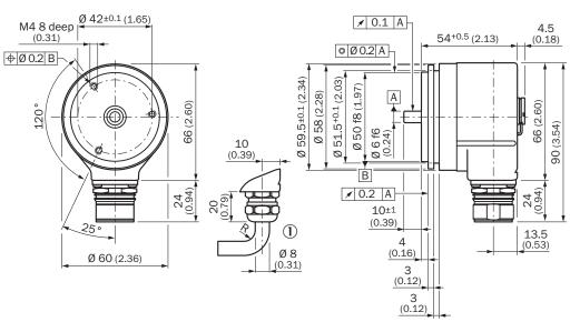
General tolerances according to DIN ISO 2768-mk ① R = min. bending radius 40 mm
