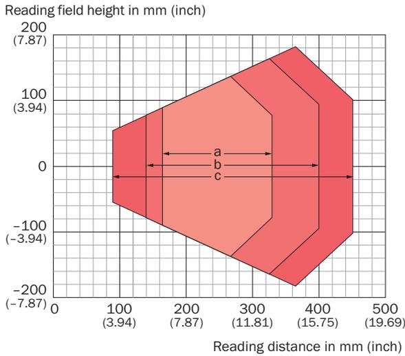
For devices with plastic reading window, the depth of field is reduced by approx. 10 %.
