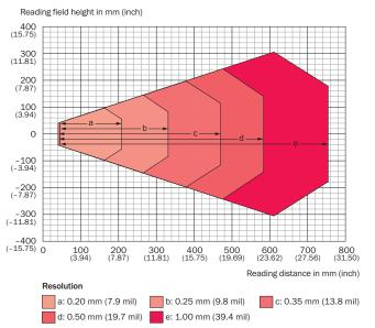
The depth of field is reduced by approx. 10% for devices with plastic lenses.
