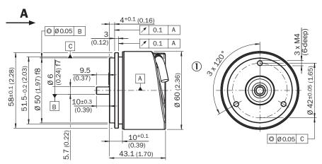
General tolerances according to DIN ISO 2768-mk  $\odot$  Cable diameter = 5.6 mm +/- 0.2 mm bend radius = 30 mm
