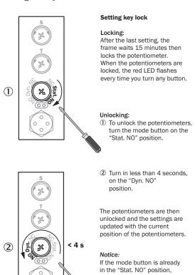
change mode previously and then apply the standard unlocking procedure.
