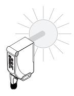
When setting the light to be detected, "1st" flashes. Press set button.
