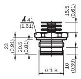
Housing with L-connector (DIN EN 175301-803 A)
