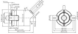
Non-tolerated dimensions according to DIN-ISO 2768-mk
