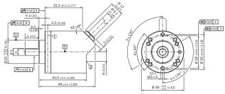
Non-tolerated dimensions according to DIN-ISO 2768-mk
