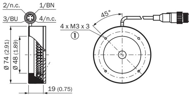
① For installation; pitch circle diameter 60 mm
