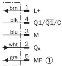
① Multifunctional input/synchronization and multiplex operation/communication Connect+
