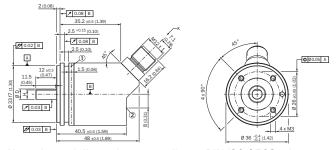
Non-tolerated dimensions according to DIN-ISO 2768-mk
