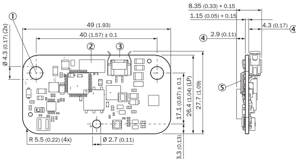
When installing/attaching the sCon® interface converter, designing the support surface as a dome is recommended. In order to guarantee the recommended distance of 1.0 mm to all electronic components from an EMC standpoint, the diameter of the domes must not exceed 8 mm. Since the sCon® interface converter can be mounted on either side, the minimum height of the domes must be 3.9 mm or 5.3 mm.
