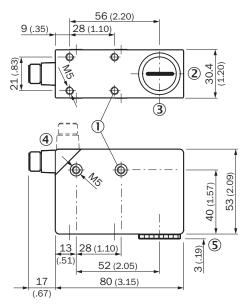
Sensing distance Sensing distance 20/50 mm
