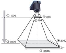
Fig. 8: Field of view V2D8512R-xxxxxxx, focal length: 12 mm
