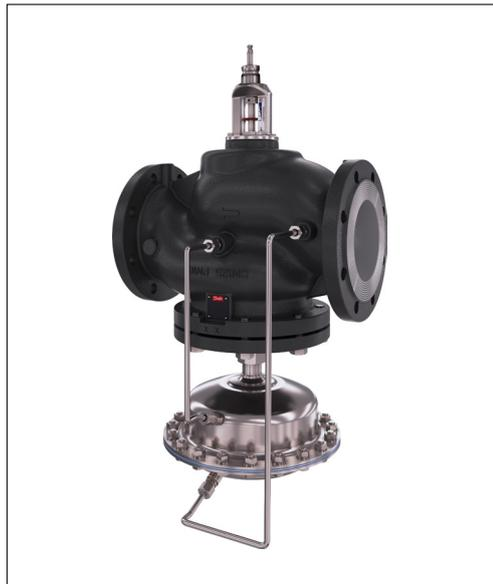
AFQM 2 is a self-acting flow controller with integrated control valve developed for the use in district heating / cooling systems. The controller prevents flow to exceed set max flow. In a combination with electrical actuators AMV(E) and ECL electronic controllers the flow and temperature can be controlled to achieve highest energy savings.
