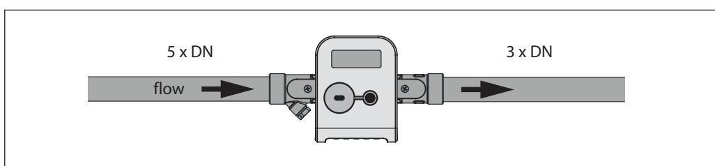
**Inlet/outlet conditions (only for DN 65 - DN 100)**
