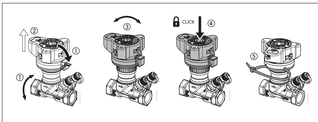
The valve has a built-in presetting feature for accurate flow ratings.
