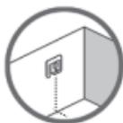
**Note for thermostat:** A floor sensor is recommended in all floor heating applications and **mandatory** to thin mats and under wooden floors to reduce the risk of over-heating the floor.
