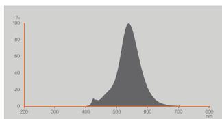
EPREL Data Spectral Diagram LEDr
