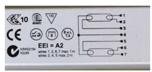
Step 2: Connect second fuse line to line "1" and "7"
