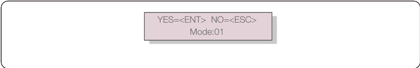
Mode "01", As shown in the figure below, the average limiting mode, the output power of each phase is the average of the three-phase load power, and it is more than the phase of the lowest power in three phases.
