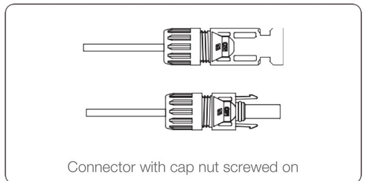
5. Measure PV voltage of DC input with multimeter, verify DC input cable polarity, and ensure each string voltage is in range of inverter operation. Connect DC connector with inverter until hearing a slight clicking sound indicating successful connection.
