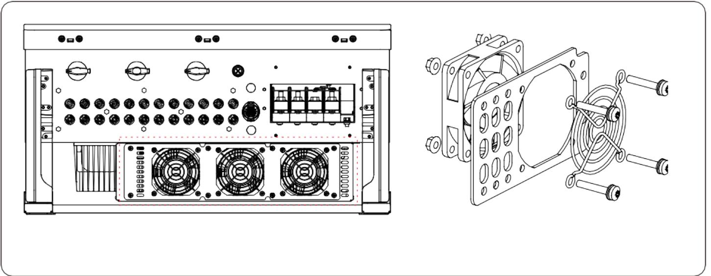
6. Disconnect the fan connector carefully and take out the fan.
