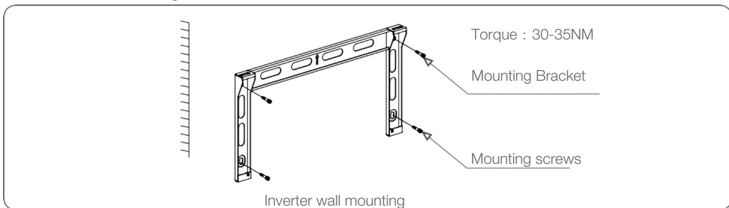
Lift the inverter and hang it on the bracket, and then slide down to make sure they match perfectly.
