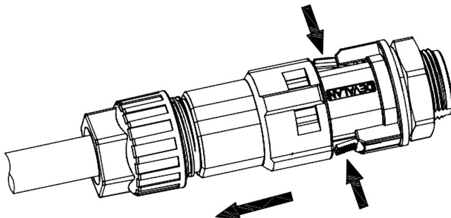
2. Use the unlock tool to insert into the groove on the sleeve and pull the sleeve to disconnect from the connector.
