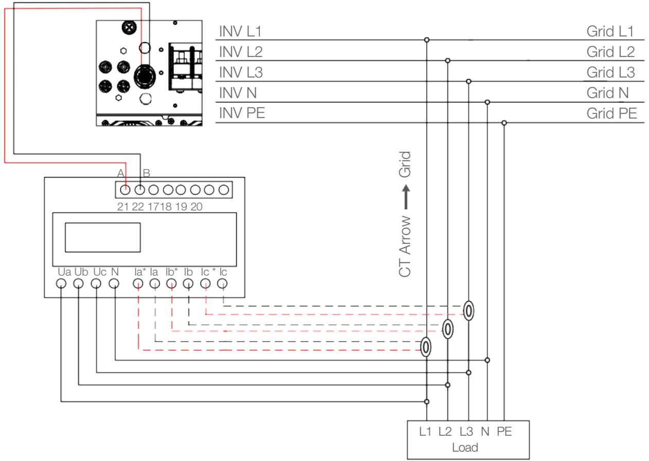
External CT Type Meter - "Meter in Load"
