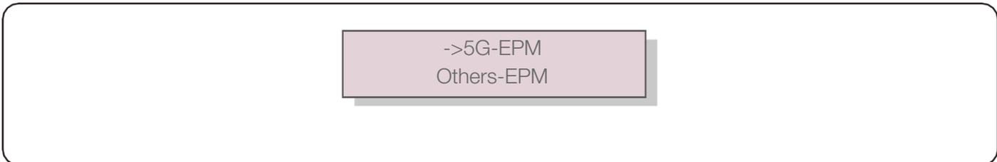
5G-EPM Failsafe Option should be turned ON when 5G series EPM device is used Others-EPM Failsafe Option should be turned ON when 2G series EPM device is used Only one option can be activated each time.
