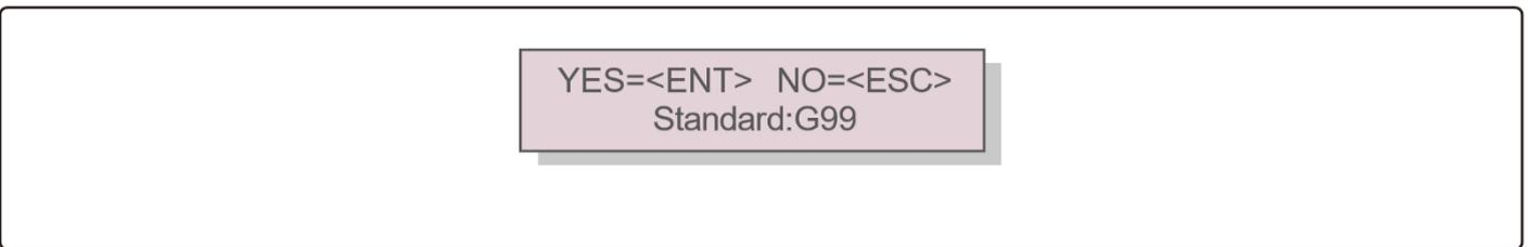
Press the UP or DOWN key to select the standard. Press the ENTER key to confirm the setting. Press the ESC key to cancel changes and return to the previous menu.
