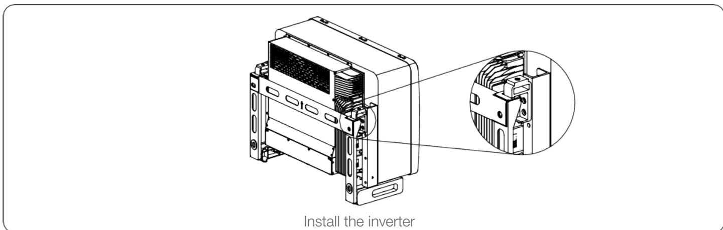
Use screws in the packaging to fix the inverter to the mount bracket.
