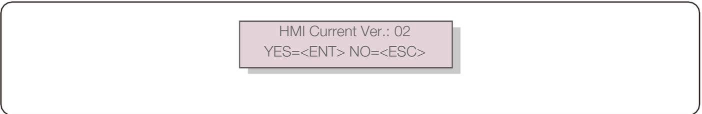
Updater is for updating LCD firmware. Press the ENTER key to start the process.
