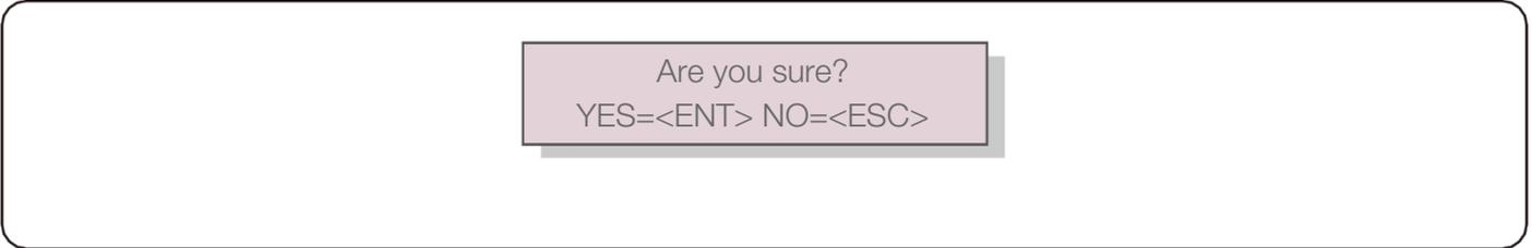
Press the ENTER key to save the setting after setting grid off.
