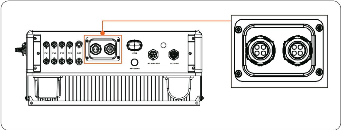
Inverter in the package is with a protective cover assembled to protect the communication ports.
