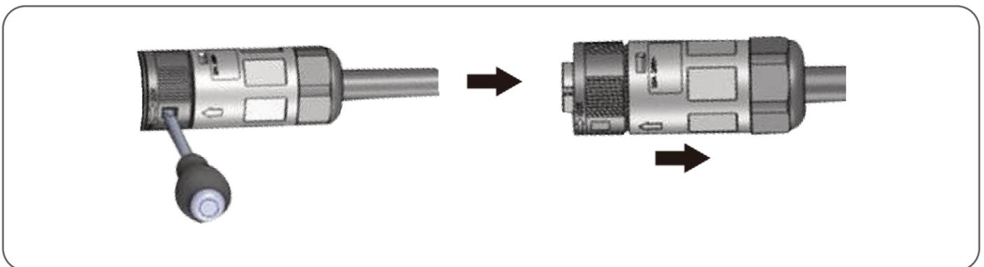
2. Disassembling body and housing for rewire.
