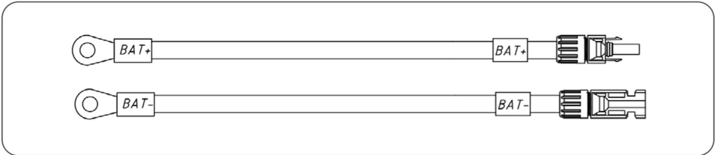
2. Connect the battery ends to the battery module positive and negative terminals.
