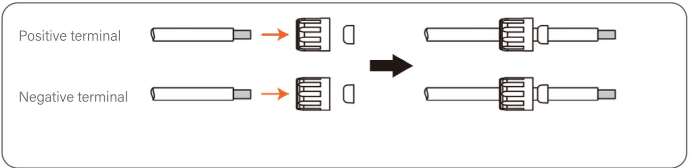
4. Connect the wire part of the DC cable to the metal DC terminal and crimp it with a special DC terminal crimping tool.
