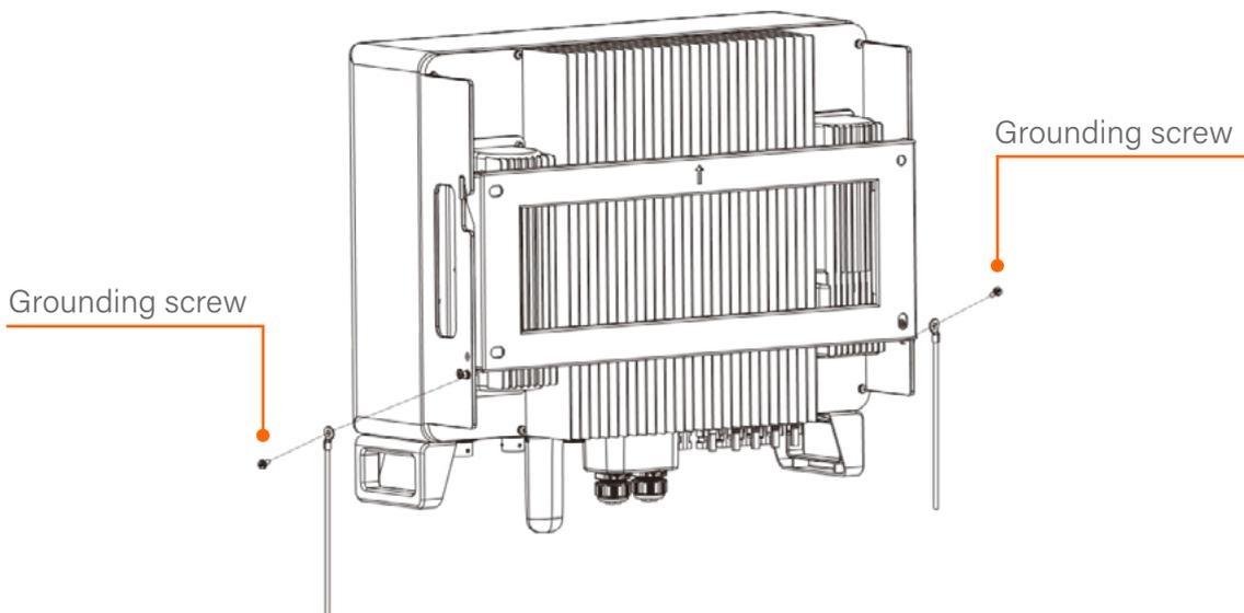
Connect the external grounding conductor
