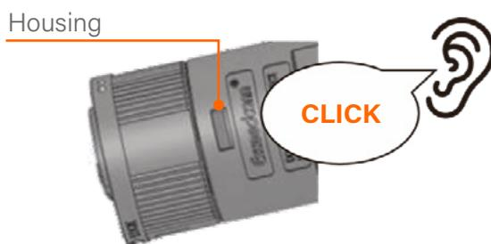
5. Insert seal body and claw into the body, and then tighten the nut with torque  $2.5\text{Nm} \pm 0.5\text{Nm}$ .
