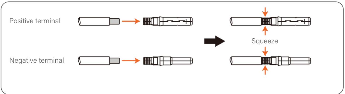
5. Insert the crimped DC cable into the DC terminal firmly, then insert the waterproof rubber ring into the DC terminal and tighten the nut.
