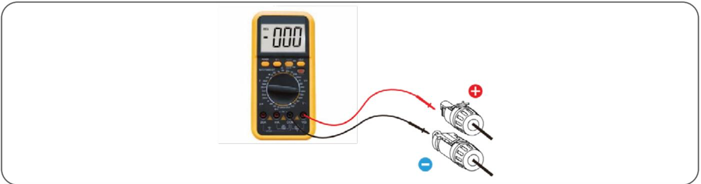
Step 2: Measure AC voltage and frequency and ensure they are within local standard.
