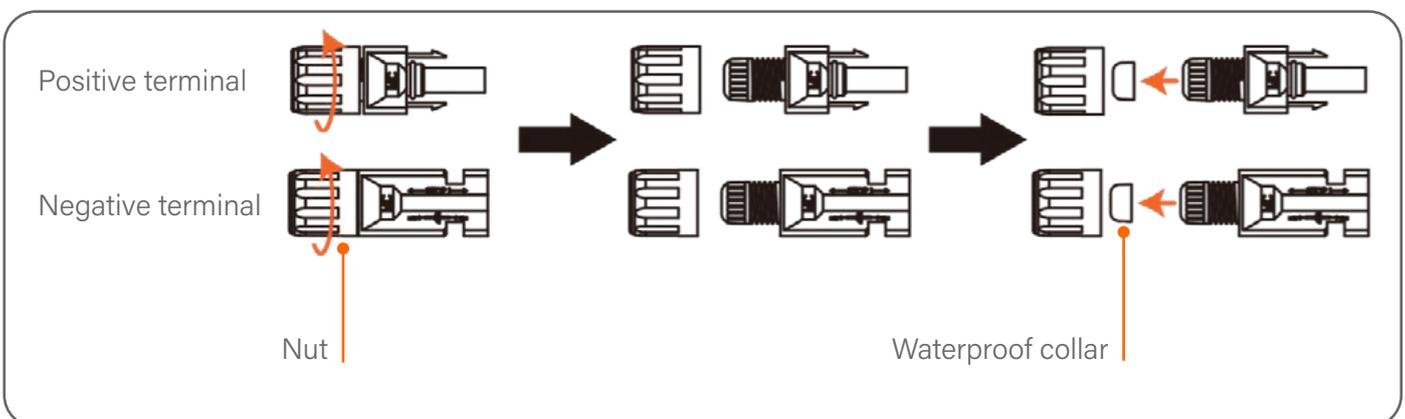
3. Pass the stripped DC cable through the nut and waterproof rubber ring.
