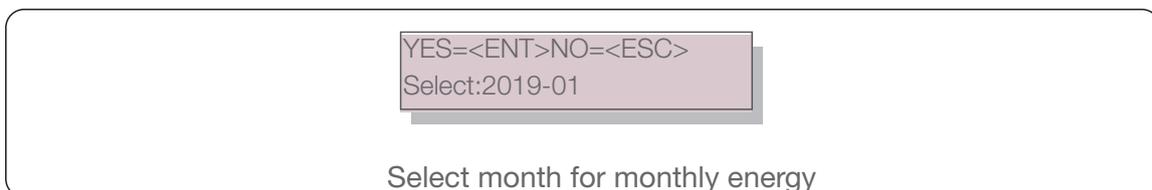
Press DOWN key to move the cursor to day and month, press UP key to change the digit. Press Enter after the date is fixed.
