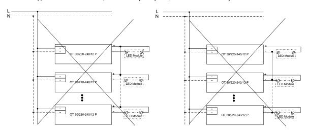
The installation of two or more OPTOTRONIC® OT 30/220-240/12 P Power supplies with common "-" or "+" wiring is forbidden.
