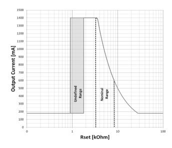
$$I_{OUT[A]} = \frac{5V}{R_{set[\Omega]}} \times 1000$$
