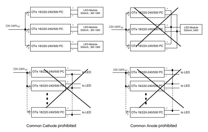
The installation of two or more OPTOTRONIC<sup>®</sup> OTe 18/220-240/500 PC Power Supplies with common "-" or "+" wiring by the intention to save wire to LED modules is prohibited, in order to avoid exceeding the maximum allowed system touch current levels on the accessible parts of the installation.
