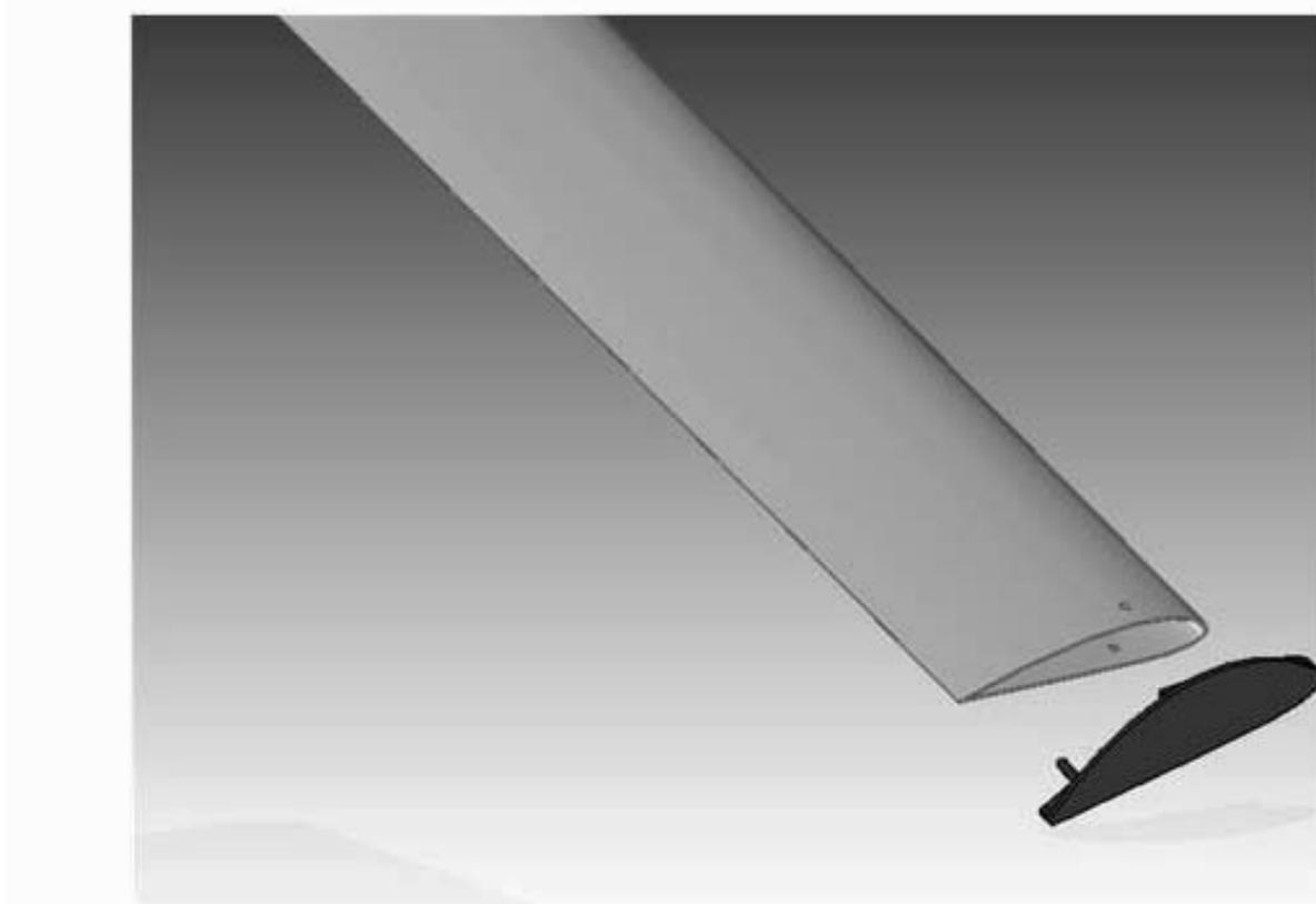
*COLOQUE EL TERMINAL DE LA PALA EN EL ASIENTO DE LA MISMA PALA
