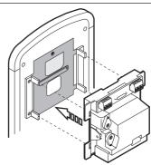
Remove the extractable terminal strips from the TV camera unit module and connect these to the respective conductors coming from the system PANELS
