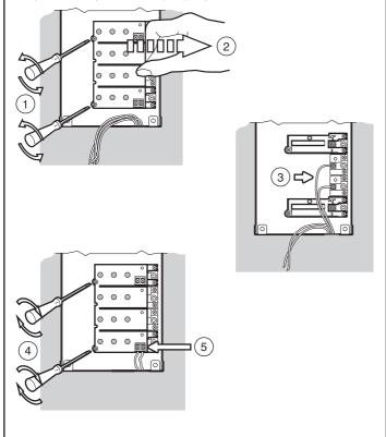
• Fasten the door unit and the camera (where relevant) to the front frame; make the electrical connections required.
