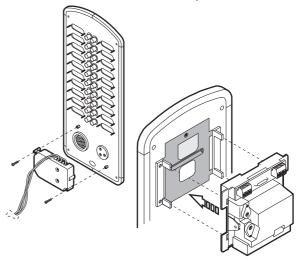
Fasten the front to the embedding box with the security screws and washers provided.
