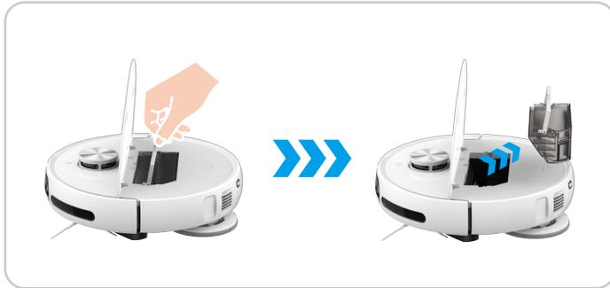
2. Unfasten the buckle on the side of the dust box, open the dust box cover and pour out the garbage inside of it.
