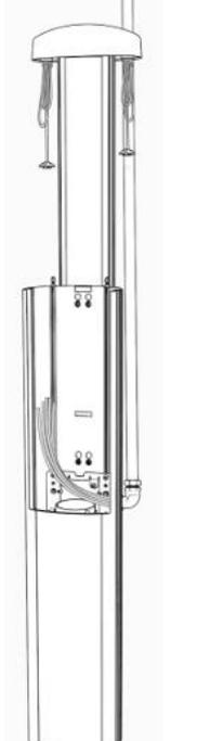
Figure 4 : raccordement borne murale
