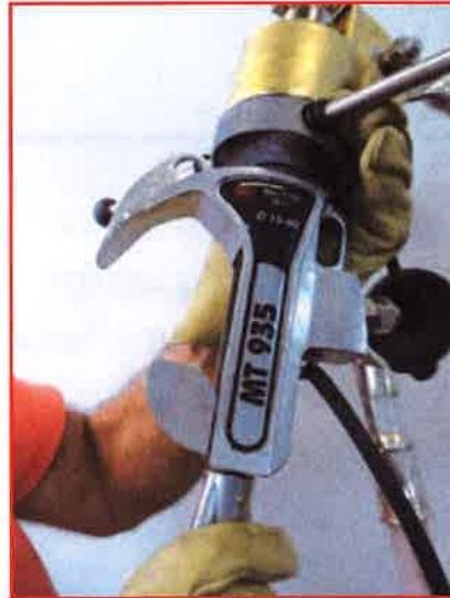
**2.** Place the earth clamp onto the earthing point.
