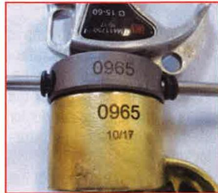
**THE INTERLOCKING IS UNIQUE. CONDUCTOR CLAMPS AND EARTH CLAMPS SHOWING DIFFERENT NUMBERS CANNOT BE INTERLOCKED.**
