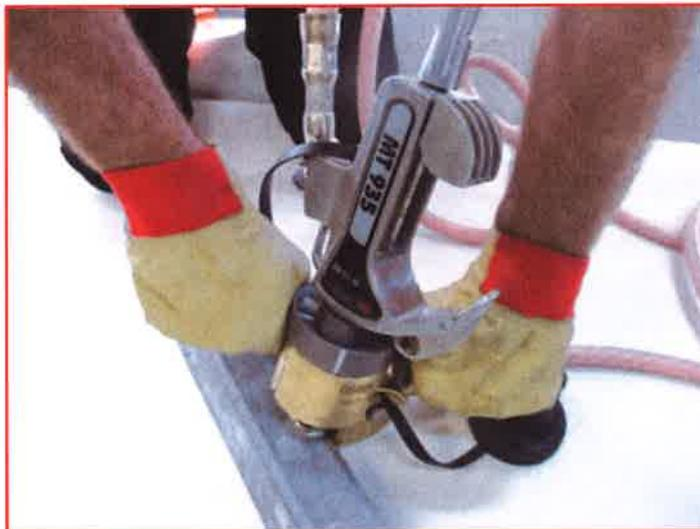
**3.** • Attach the earth clamp by screwing it on, turning clockwise the operating lever.
