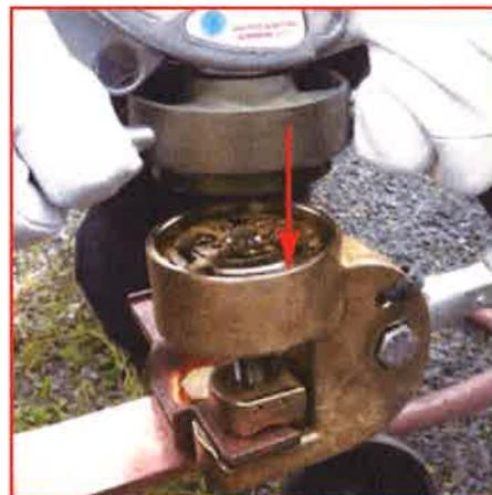
**3.** • Unscrew the earth clamp by turning the lever anticlockwise. Apply balanced effort using both hands along the axis of the clamp.
