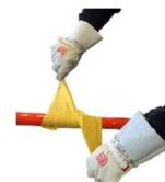
**MO-984:** Silicone rag to maintain the insulating properties of the stick. It is necessary to clean and dry the surfaces before using the rag.
