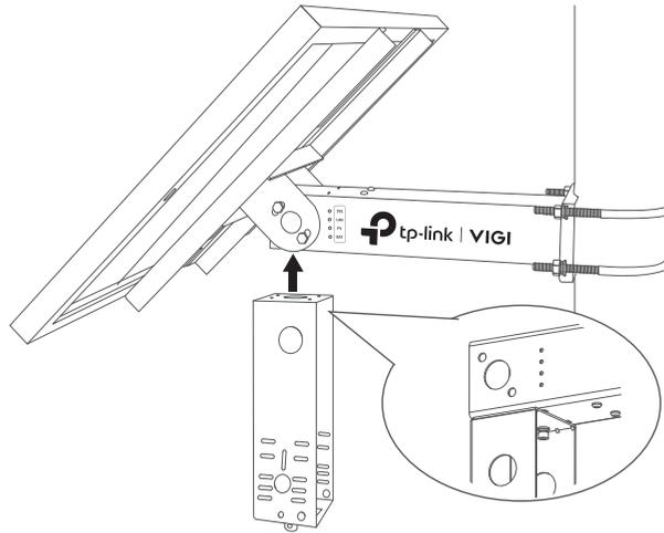
2. Install devices on the vertical mount. Different types of mounts have varying access methods, and the corresponding type of bracket should be selected for installation according to the actual situation of the device.
