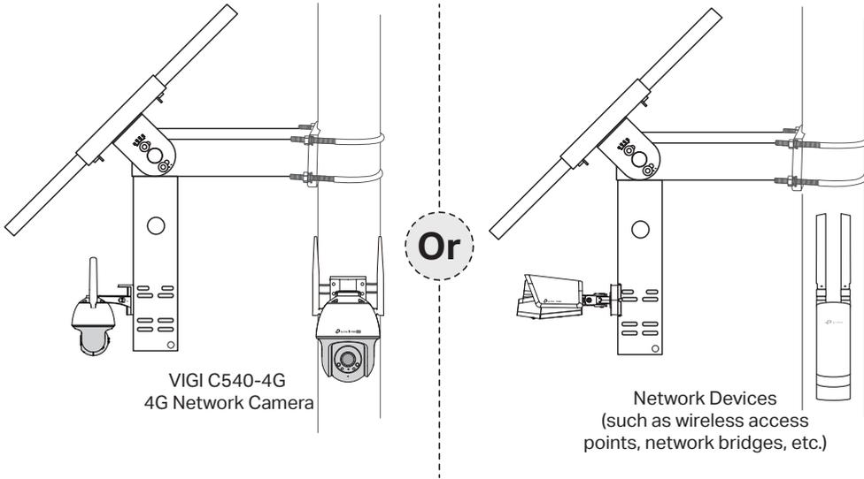
**Step 1. Connect the RJ45 network interface of the solar panel to the network devices (such as access points, bridges, and 4G cameras).**
