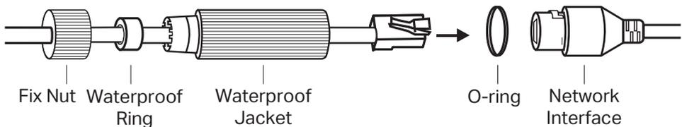
1. Route the network cable through the following components in order: fix nut, waterproof ring, and then the waterproof jacket.
