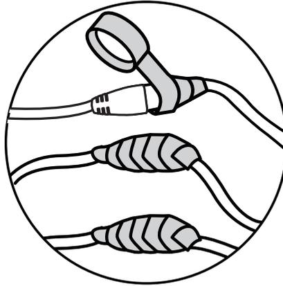
**Note:** When using waterproof tape, wrap the first layer, then cut. Apply a second layer, ensuring no gaps between the connection and tape for secure waterproofing.
