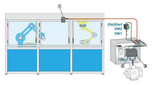
1 XCSRC•3M12: XCSRM RFID Safety Switch advanced model
