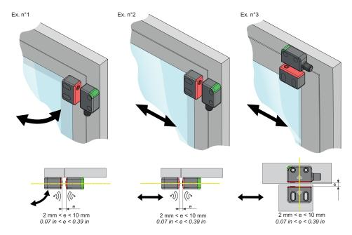
e Recommended minimum mounting distance between actuator and switch.
