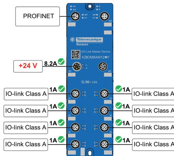
One IO-Link class A device each requiring maximum 1 A current is connected to the ports X1 to X8 of XZIOM8AM12PY. XZIOM8AM12PY, requires 0.2 A current.
