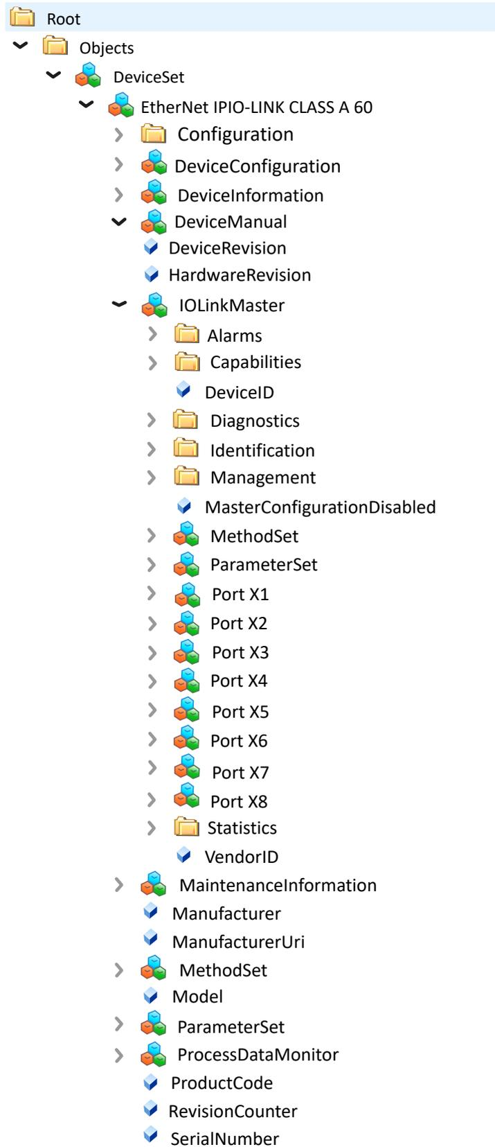
The following figure shows a part of the information model of the IO-Link port:
