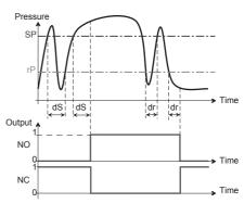
The Time Delay (see  $\mbox{\bf dS}$  and  $\mbox{\bf dr}$  menu) is typically used to filter out the fast pressure transients.
