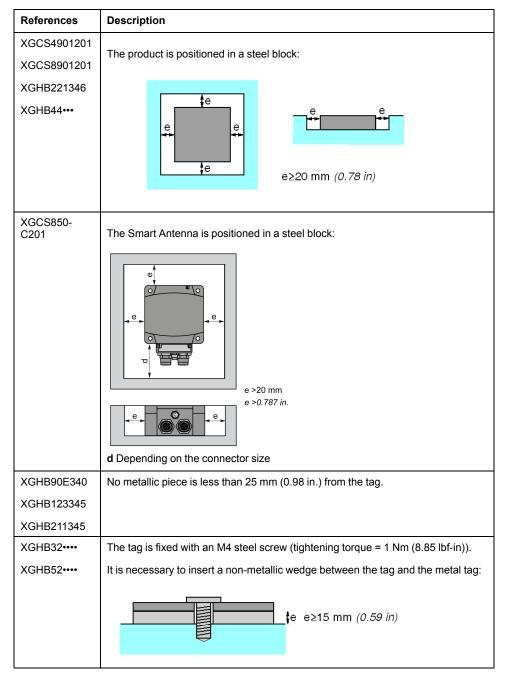
The table shows the effect on the nominal sensing distance when the Smart Antenna and the tag are assembled in metal according to the most unfavorable cases shown above:
