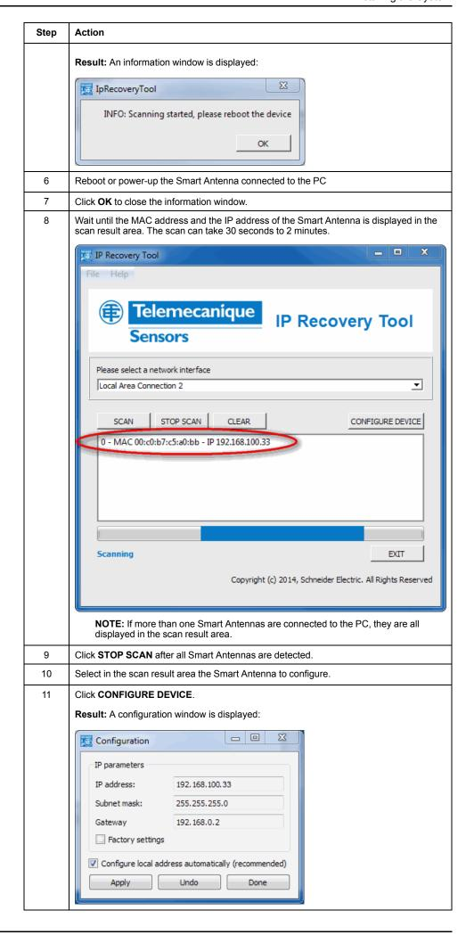
Installing the System Ethernet Smart Antenna
