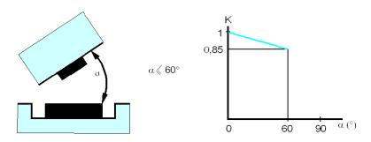
K = correction factor to be applied to the nominal sensing distance.
