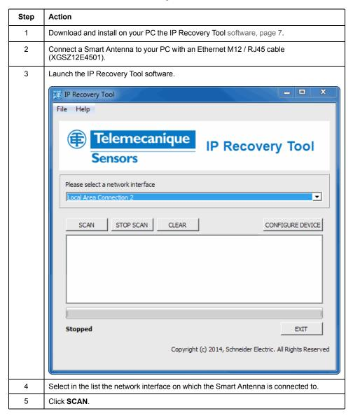
Ethernet Smart Antenna Installing the System
