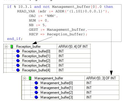
**NOTE:** The ADDR function is structured: '(XWAY address)Rack.Module. Channel.Modbus address)'.
