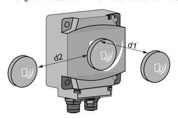
Minimum distances between 2 identical tags according to their positioning:
